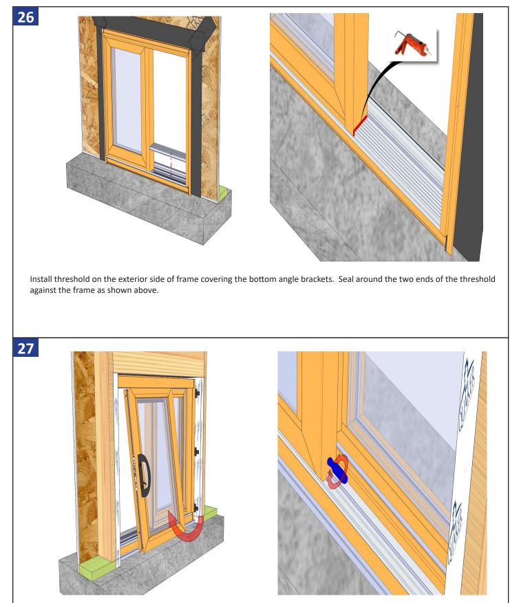
Angle the active panel with the top inserted into the head track, and then lift and set the bottom rollers on the roller track. Adjust the rollers as needed to insure the panel is level, square, and slides smoothly.
