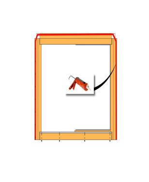
Apply a continuous 3/8" diameter bead of sealant along the backside of the nailing flange. Bead must run around both sides and across the head, in line with and completely covering the nail flange holes.
