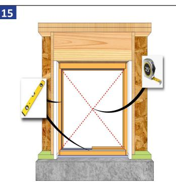
Check that the door is square. Adjust shims as needed until diagonal measurements are within 1/8''. Level at the sill and plumb the frame.
