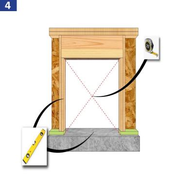
Check that the opening is square. The diagonal measurements need to be within 1/8" of each other. Verify the rough opening is plumb and level. The sill plate beneath the unit must be level for proper unit operation.
