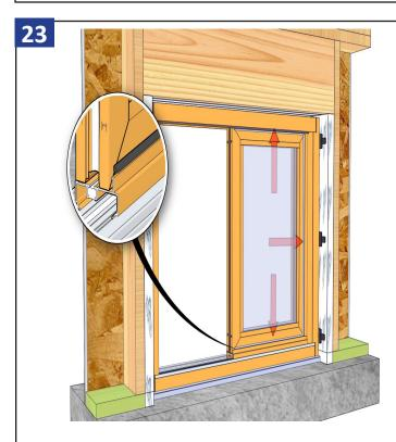
Install wedge gaskets in the sill, head, and jamb around the interior of the frame and panel to secure the panel in place.
