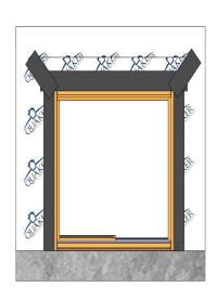
Unfold the house wrap top flap and tape the angled seams as shown.
