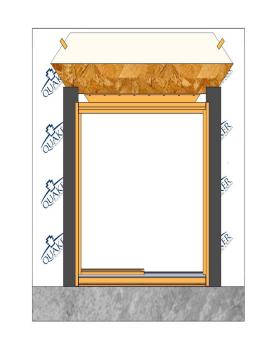
Apply flashing tape at the sides of the door as shown. Smooth using a J-roller. Extend tape a minimum of 2" pass window frame.
