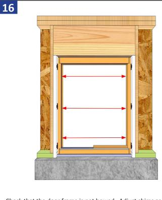
Check that the door frame is not bowed. Adjust shims as needed until measurements are within 1/8". Finish fastening the unit every hole or a minium of 12" on center.
