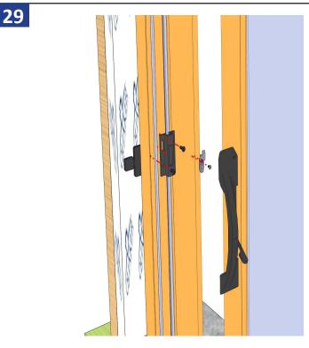
Install jamb lock keepers for the active panel and screen door.
