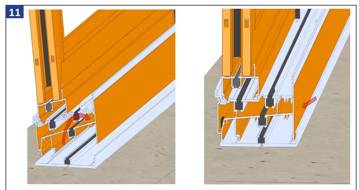
Center and set the door frame into the rough opening, making sure there are equal gaps on both sides of the door. Angle the door frame with the top tilted out, and set the exterior sill frame inside the exterior leg of the sub-sill anchor plate as shown above. Push the frame in against the framing to lock the sill into the sub-sill anchor plate.
