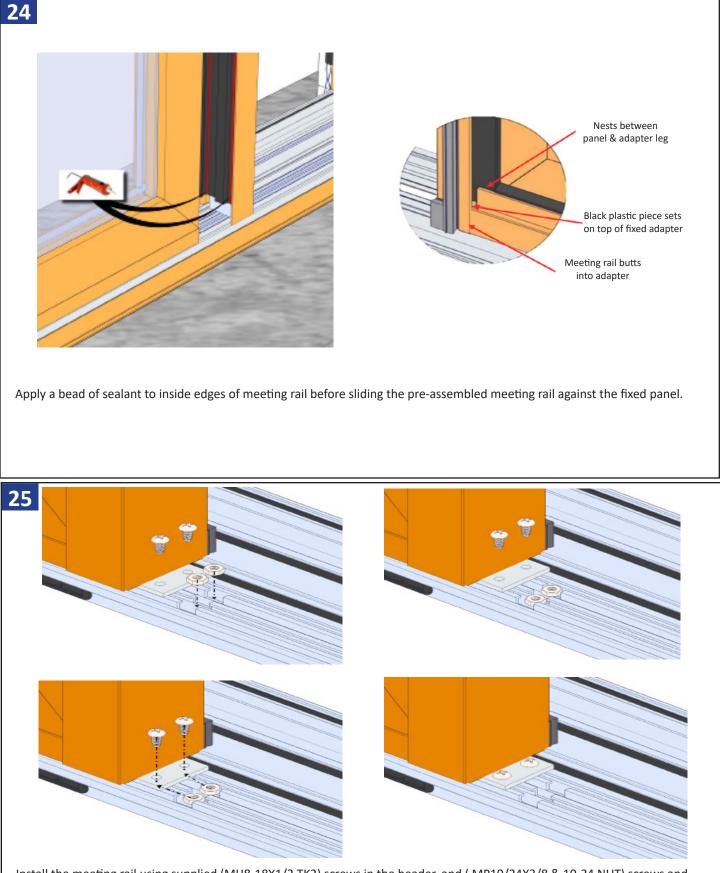
Install the meeting rail using supplied (MH8-18X1/2 TK2) screws in the header, and (MP10/24X3/8 & 10-24 NUT) screws and nuts in the sill angle brackets.
