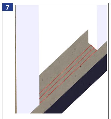
Apply three 3/8" continuous beads of sealant across the entire width of the rough opening sill, and a 3/8" continuous bead of sealant 1/2" from each side of opening as shown above.
